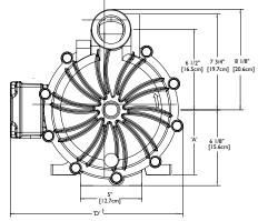
Also available 2 x 2 or 3 x 2 150 lb. ANSI/ISO PN20/PN40/ JIS 10K or 63mm x 63mm union connection. Flanges are in compliance with bolting dimensions only.
